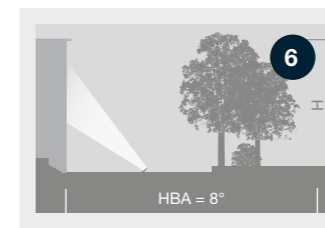
RS08 – for illuminating objects, buildings and arenas
