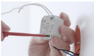
01 Connect the DALI PCU to the mains and DALI wires.
